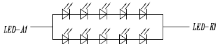
Figure : LED connection of backlight
